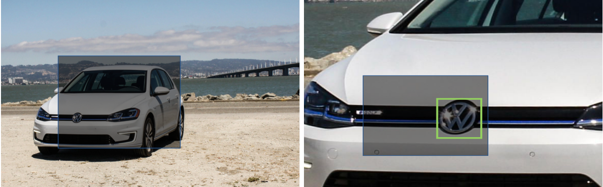
Figure 7.11: A single receptive field such as that of the RPN cannot match the object scale variability. This is also an example where our detector was not able to detect the logo due to small size but was later succeeded after doing up-sampling.
